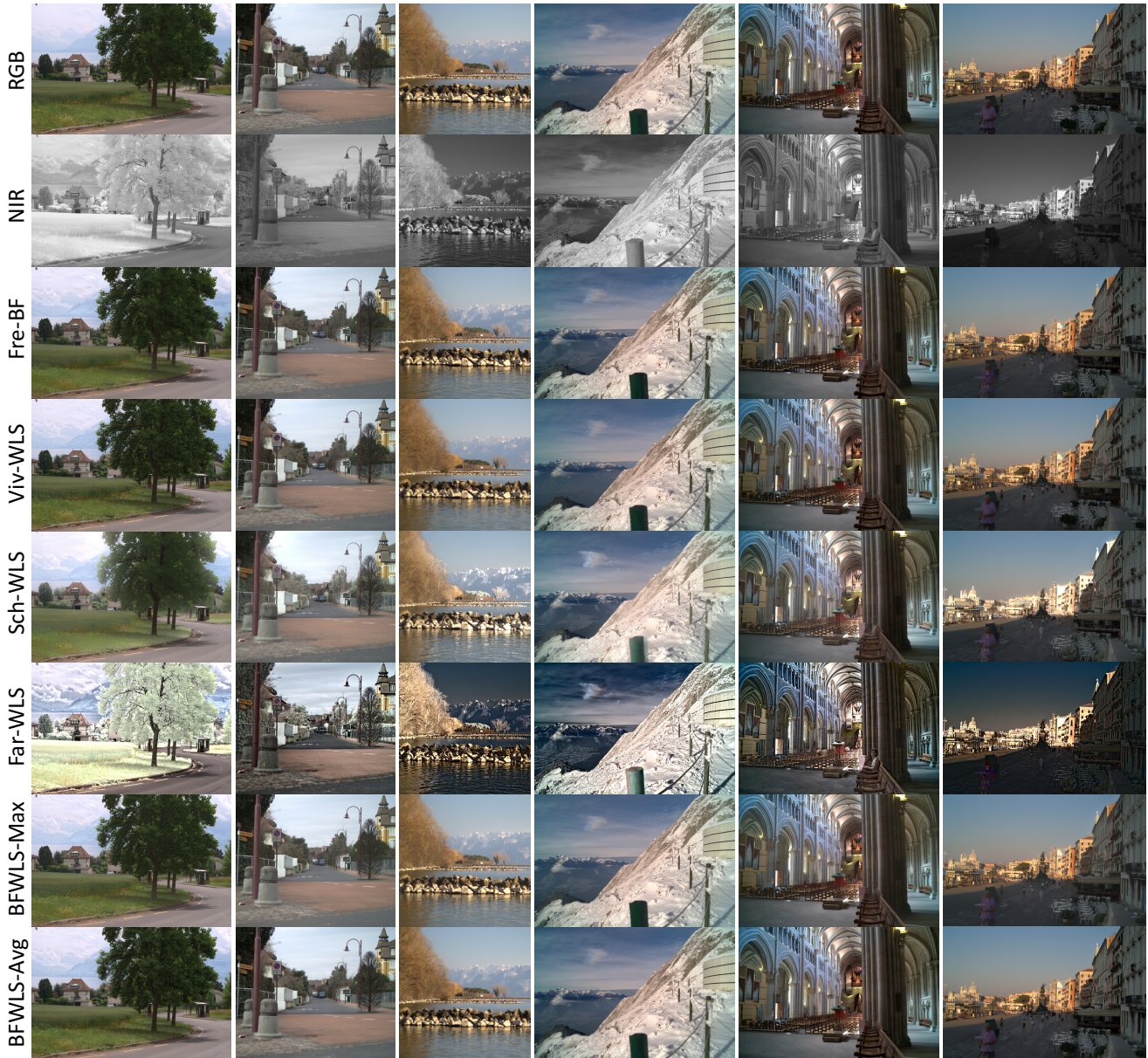
Figure 4: Visual comparison of BFWLS against state-of-the-art algorithms for RGB-NIR image fusion. In the zoomed-in view, note how BFWLS-Avg adapts well to the local structures and details when compared to the other methods. Best viewed in color.
